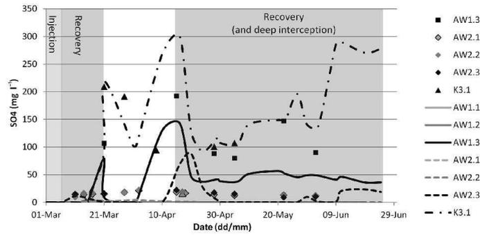
Figure 9. Modeled and observed SO<sub>4</sub> concentrations at the most relevant well screens.
