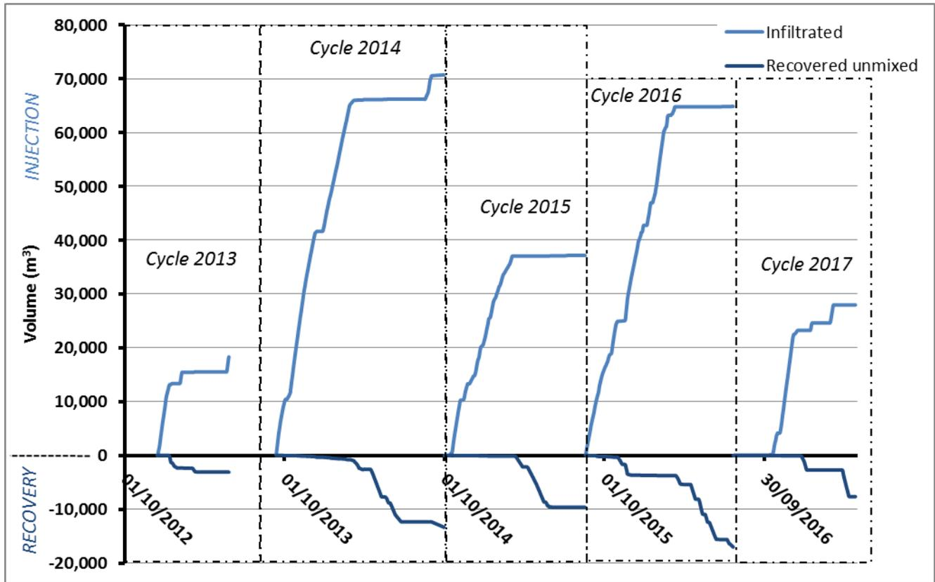
Figure 12: Infiltrated and recovered volumes per cycle versus time (data on a daily basis)
