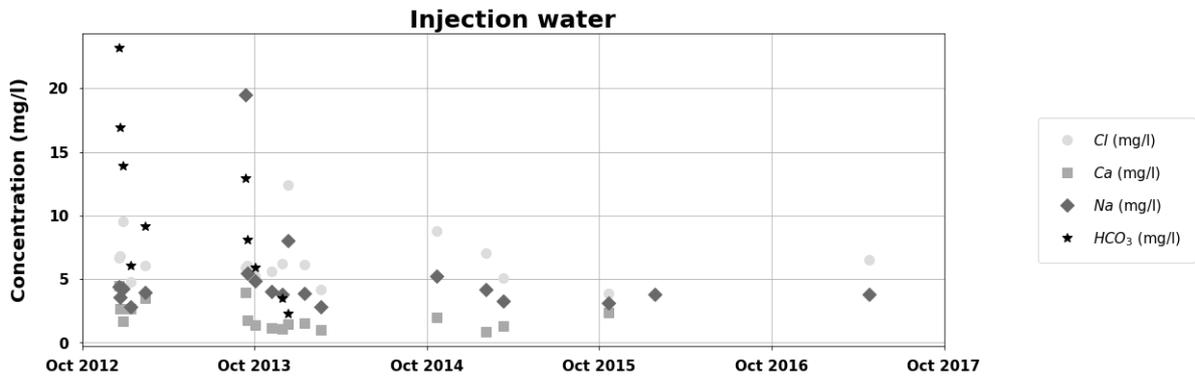
Figure 31: Concentrations of Cl, Ca, Na, and HCO<sub>3</sub> in the freshwater used for infiltration at ASRRO Westland.
