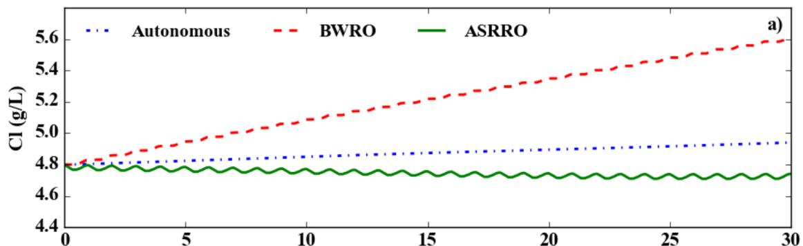
Figure 33: Overage concentrations of chloride in the Westland groundwater system during 30 years based on groundwater modelling assuming an autonomous case (no groundwater use), use of BWRO (current situation), and ASRRO (approach developed in DESSIN).
