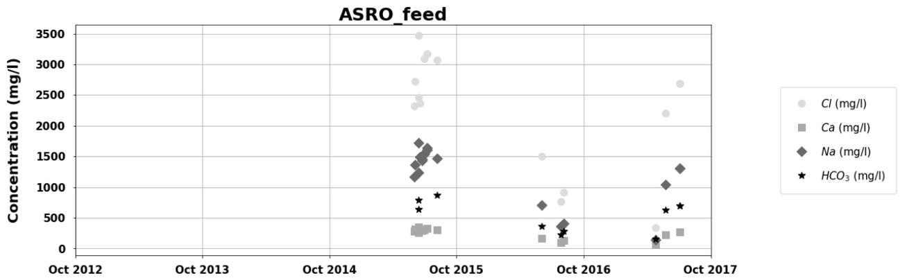
Figure 41: Concentrations of Cl, Ca, Na, and HCO<sub>3</sub> in brackish groundwater intercepted to feed the ASRRO-system.
