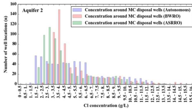
**Figure 8.** Distribution of local chloride concentrations in the 50 m × 50 m model cells of the MC disposal wells (Aquifer 2) of each individual BWRO and ASRRO system (average during the final year (year 30)).
