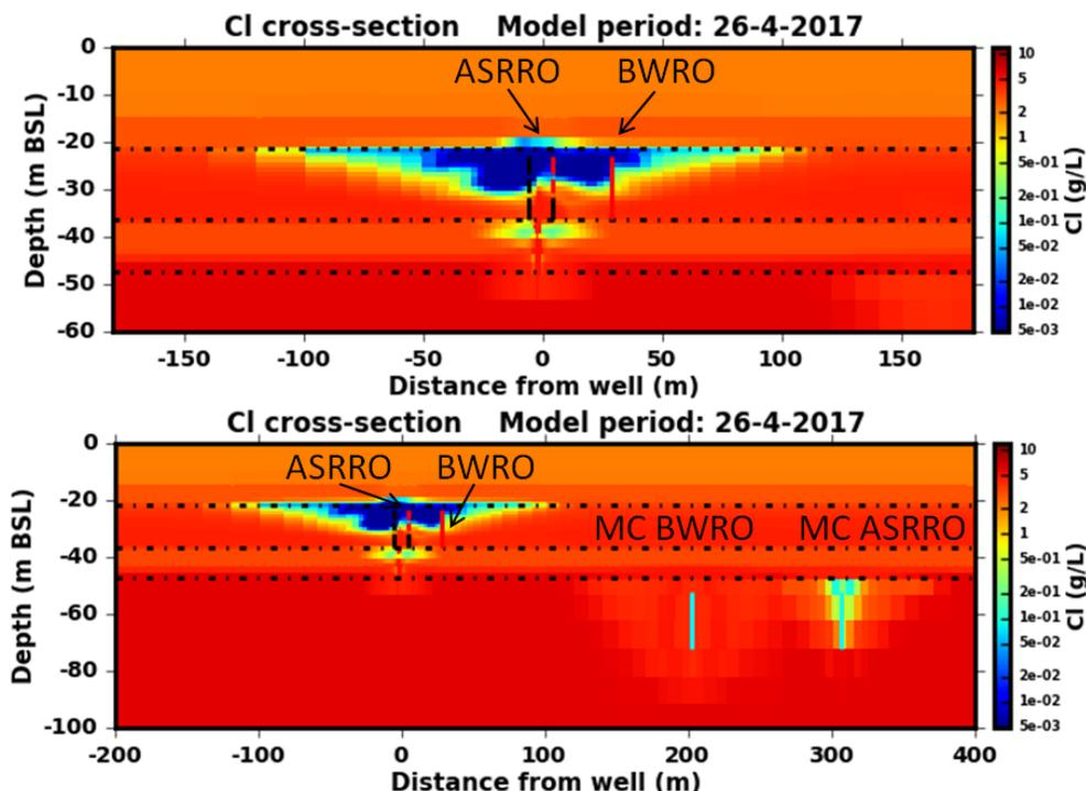
Figure 29: Final modelled chloride concentrations (26 April 2017) for cross-sections through the ASRRO wells (AW1 and AW2), both near the ASRRO (top) and an overview including membrane concentrate injection wells (bottom).
