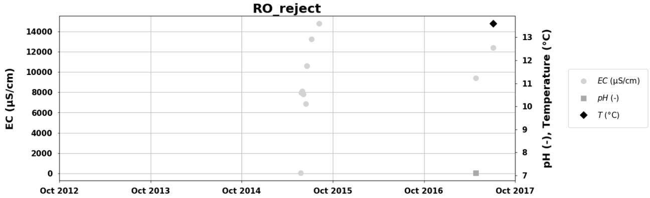
Figure 43: Electrical conductivity (EC in  $\mu\text{S}/\text{cm}$ ), pH (-), and temperature (Temp in  $^{\circ}\text{C}$ ) of brackish groundwater rejected by the BWRO-system.
