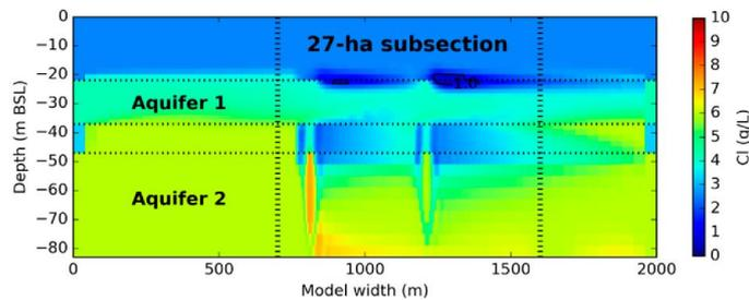
**Figure 5.** Chloride concentrations along the mirror plane (W- > E) of Local Model where the MC disposal wells are situated (scenario ASRRO;  $t = 30$  year, end of summer). The 27-ha model subsection includes the part shown between the vertical dotted lines ( $x = 70$ ;  $x = 160$ ).
