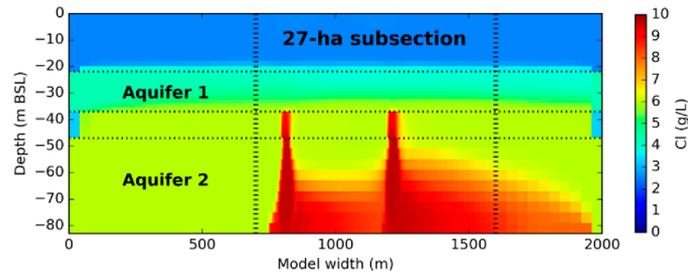
**Figure 6.** Chloride concentrations along the mirror plane (W- > E) of the Local Model where the MC disposal wells are situated (scenario BWRO;  $t = 30$  year, end of summer). The 27-ha model subsection includes the part shown between the vertical dotted lines ( $x = 70$ ;  $x = 160$ ).
