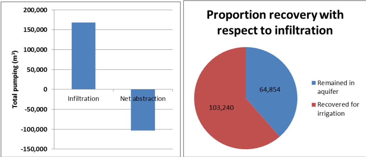
Figure 11: Total freshwater infiltration in and abstraction from the Westland target aquifer at the Westland demo site (left, 'net abstraction' = the production of freshwater from the aquifer by direct recovery of rainwater or *after* RO-treatment) and the resulting water balance (right). Based on three complete cycles (2014 – 2016).
