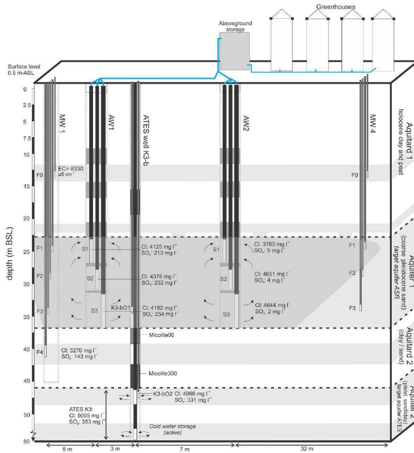
**Figure 1.** Cross section of the Westland ASR site to schematize the geology, ASR wells, ATEs well, and the typical hydrochemical composition of the native groundwater. Horizontal distances not to scale.
