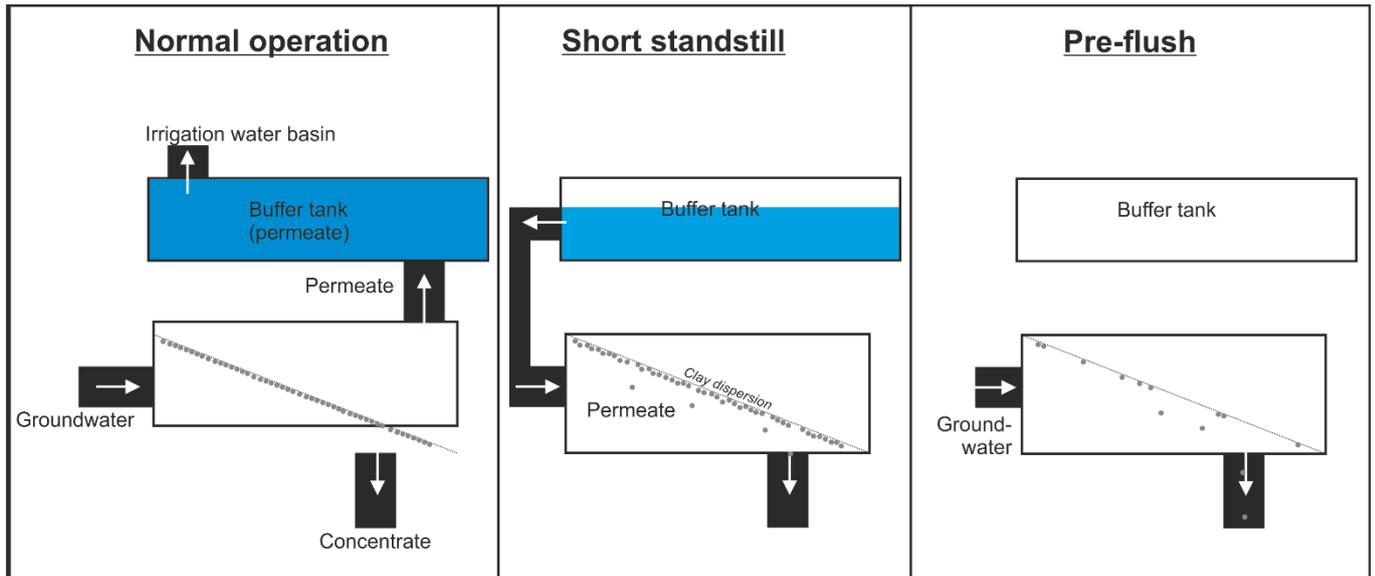
Figure 19: Flushing of the BWRO membranes as frequently applied in 2016 to clean the membrane.
