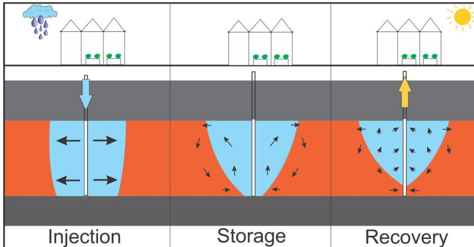
Figure 3: Freshwater loss during ASR in brackish and saline aquifers due to buoyancy effects.
