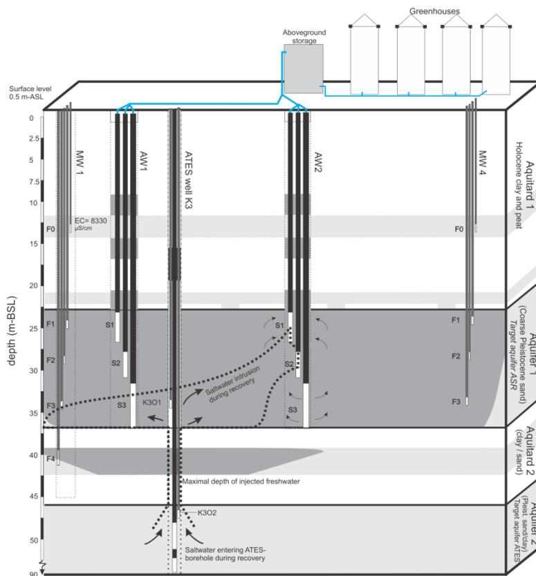
Figure 10: Leakage of deep, saline groundwater during recovery, hampering optimal recovery of freshwater from the Westland target aquifer.
