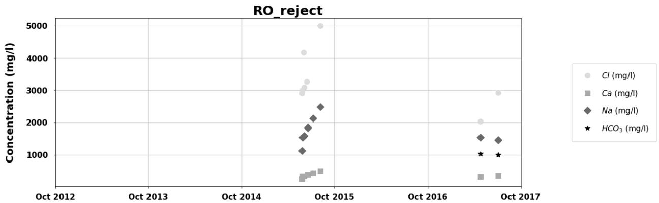
Figure 44: Concentrations of Cl, Ca, Na, and  $\text{HCO}_3$  in brackish groundwater rejected by the BWRO-system.
