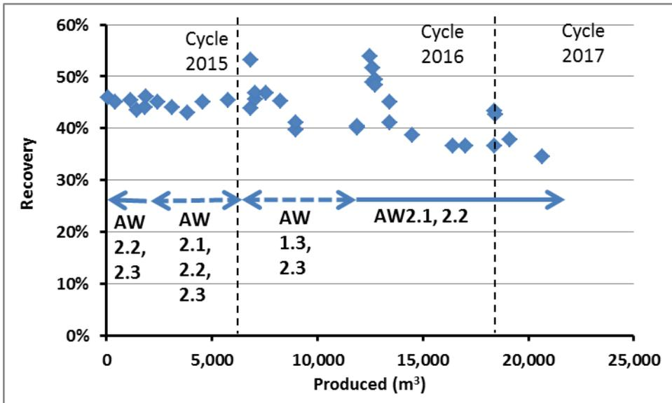
Figure 14: RO-recovery (percentage of abstracted water transformed to freshwater) of the ASRRO-plant
