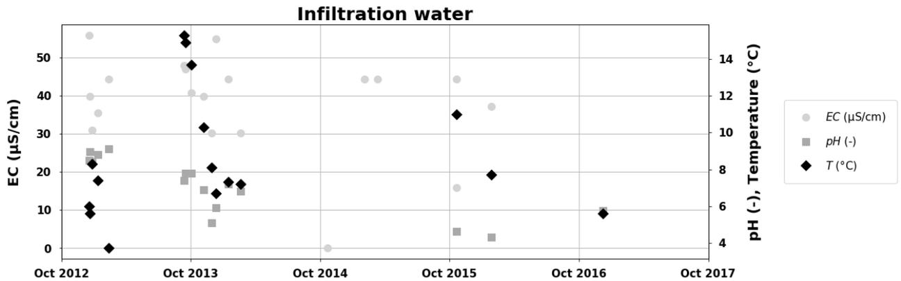
Figure 30: Electrical conductivity (EC in  $\mu\text{S}/\text{cm}$ ), pH (-), and temperature (Temp in  $^{\circ}\text{C}$ ) of the freshwater used for infiltration at ASRRO Westland.
