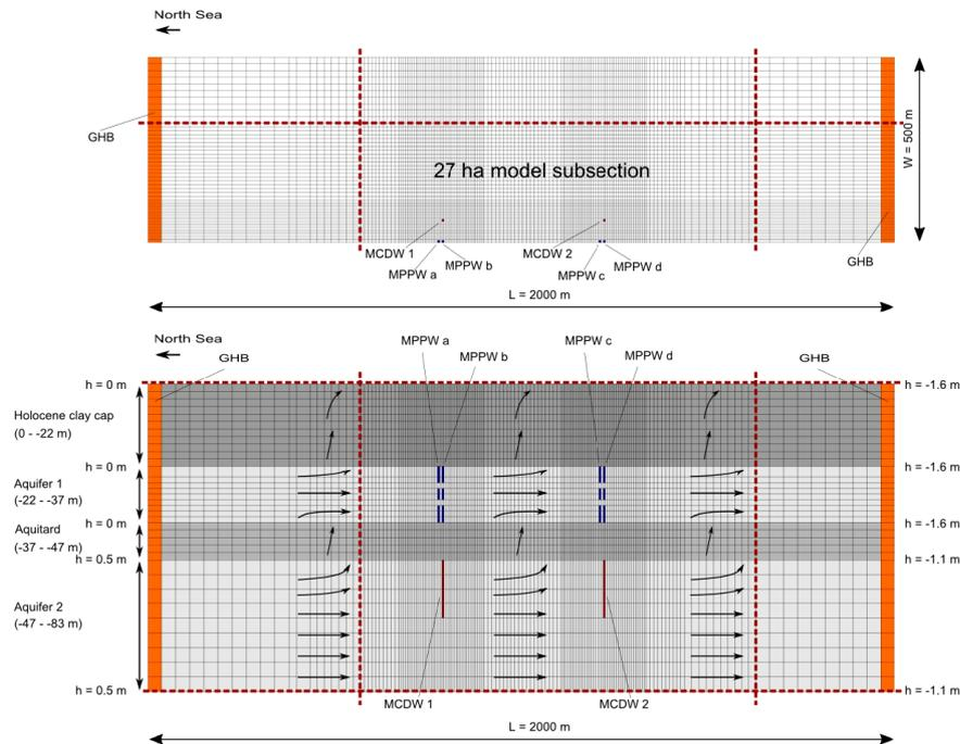
**Figure 3.** Top: Top view of the Local Model grid. Bottom: Cross-sectional view (West-East) showing the hydraulic heads ( $h$ ) and the expected flow pattern through the various geological layers for the autonomous situation. The 27-ha subsection (area of the greenhouses connected to the ASRRO system) of the model is located within the marked box. The vertical exaggeration is 10:1.
