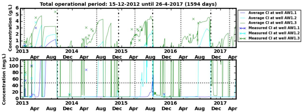
Figure 49: Measured (crosses) and modelled (solid lines) chloride concentration in water in the different well screens of the ASR-well (AW1) at Westland from 15 December 2012 until 26 April 2017. The black dotted and dashed vertical lines indicate the start of the infiltration and recovery period respectively. The horizontal dashed line in the bottom graph represents the maximum allowable concentration limit of chloride upon abstraction.
