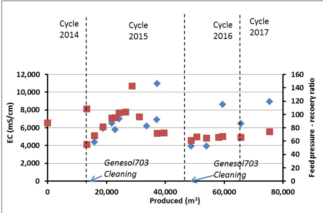
Figure 21: The feed pressure – recovery ratio (red) and the observed ECs (blue) of the feedwater during sampling at the BWRO plant.
