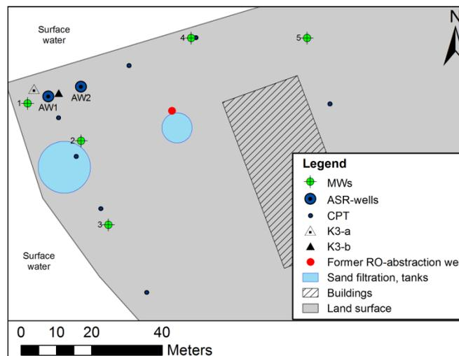
Figure 8: Locations of ASR (AW), ATES, and monitoring wells (MW). The former RO abstraction well is used during the DESSIN pilot to abstract mixed rainwater / groundwater at the fringe of the freshwater bubble and use this for desalination with the 'BWRO' plant.
