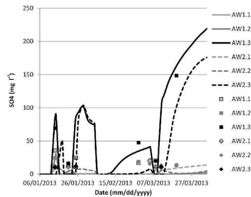
**Figure 7.** Modeled (solid lines) and observed (data points) SO<sub>4</sub> concentrations. Borehole leakage at the location of the current ATEs K3 well via a 1 m × 1 m borehole with  $K = 1000 \text{ m d}^{-1}$ . High concentrations indicate admixing of deeper saltwater. Observed SO<sub>4</sub> concentrations become in line with the modeled concentrations.
