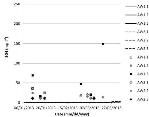
**Figure 6.** Modeled (solid lines) and observed (data points) SO<sub>4</sub> concentrations without borehole leakage. High concentrations indicate admixing of deeper saltwater. Observed SO<sub>4</sub> concentrations by far exceed the modeled concentrations.
