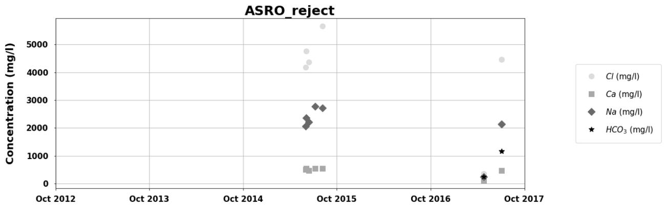
Figure 47: Concentrations of Cl, Ca, Na, and HCO<sub>3</sub> in brackish groundwater rejected by the ASRRO-system.
