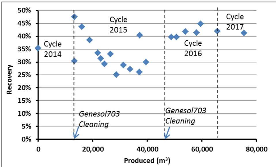
Figure 16: Recovery (percentage of abstracted water transformed to freshwater) of the BWRO-plant
