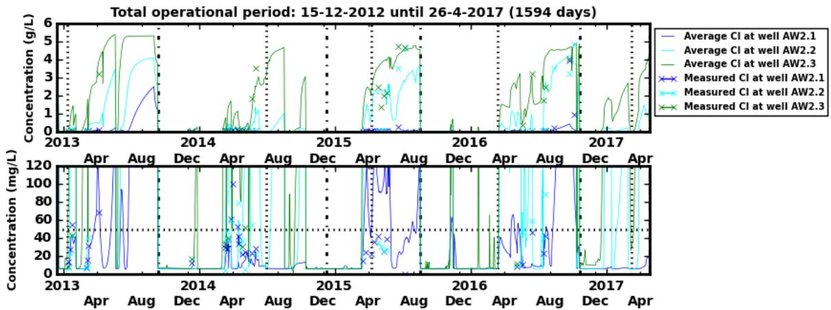
Figure 50: Measured (crosses) and modelled (solid lines) chloride concentration in water in the different well screens of the ASR-well (AW2) at Westland from 15 December 2012 until 26 April 2017. The black dotted and dashed vertical lines indicate the start of the infiltration and recovery period respectively. The horizontal dashed line in the bottom graph represents the maximum allowable concentration limit of chloride upon abstraction.
