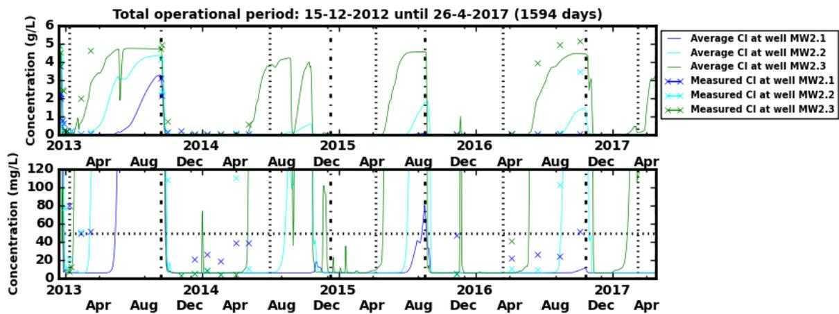
Figure 52: Measured (crosses) and modelled (solid lines) chloride concentration in water in the different well screens of the monitoring well (MW2) at Westland from 15 December 2012 until 26 April 2017. The black dotted and dashed vertical lines indicate the start of the infiltration and recovery period respectively. The horizontal dashed line in the bottom graph represents the maximum allowable concentration limit of chloride upon abstraction.
