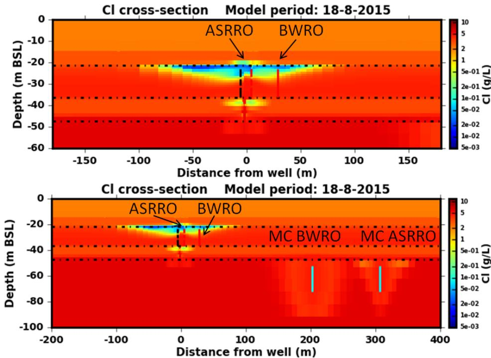
Figure 28: Modelled chloride concentrations after a prolonged period of abstraction (18 August 2015) for cross-sections through the ASRRO wells (AW1 and AW2), both near the ASRRO (top) and an overview including membrane concentrate injection wells (bottom).
