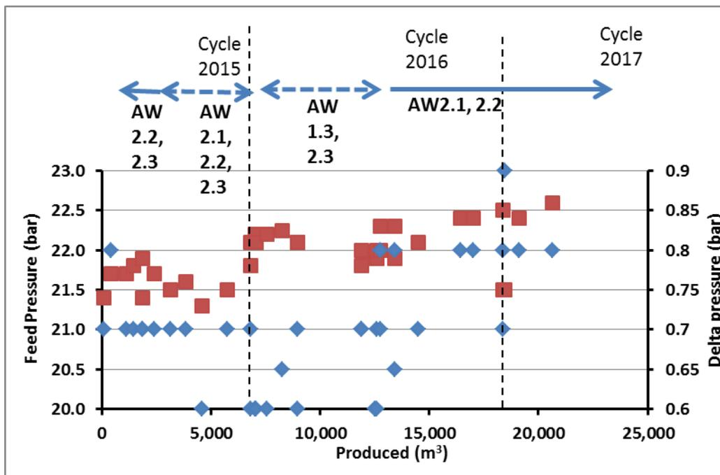
Figure 17: Feed pressure (red) and delta-pressure (blue) between feed and reject side for the ASRRO-plant.
