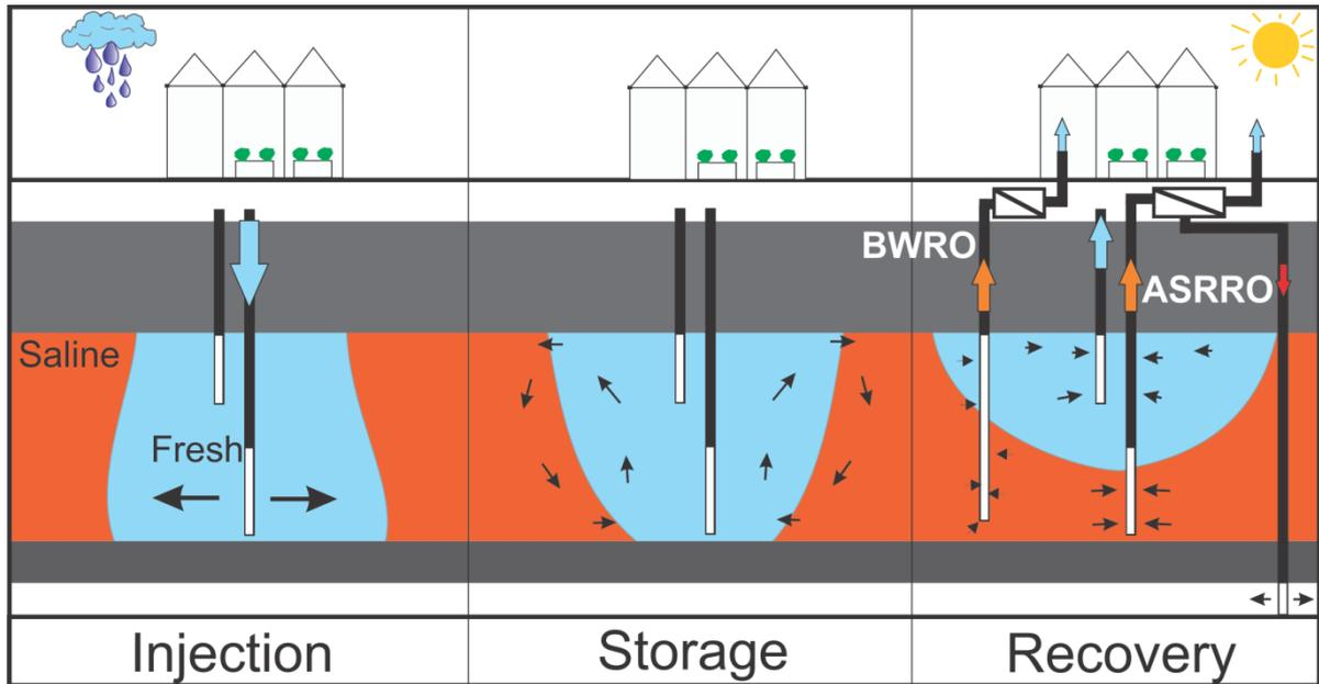
Figure 9: Abstraction of mixed rainwater / brackish groundwater via BWRO and ASRRO
