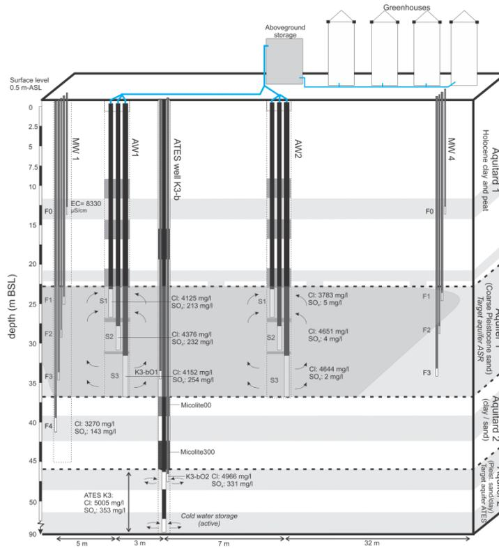
Figure 7: Cross-section of the Westland ASR site to schematize the geology, ASR wells, aquifer thermal energy storage (ATES) well, and the typical hydrochemical composition of the native groundwater. Horizontal distances not to scale.
