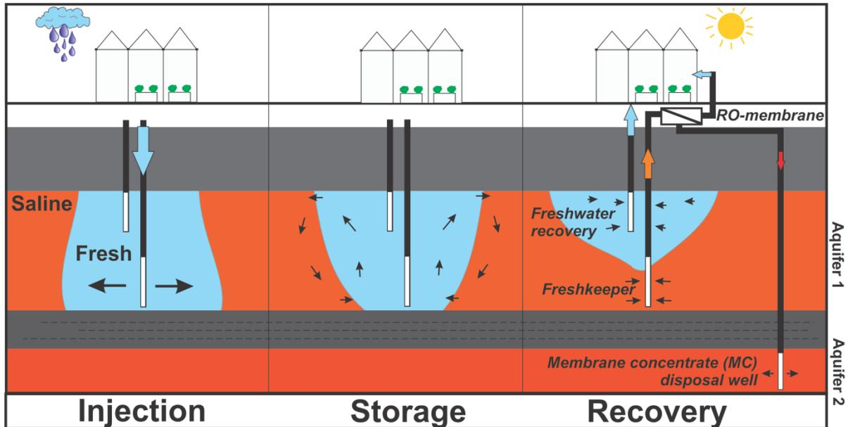
Figure 4: Operation of an ASRRO system, as realized at the Westland demo site
