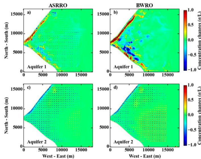
**Figure 10.** Relative chloride concentration changes (g/L) between ASRRO and Autonomous and between BWRO and Autonomous after 30 years in Aquifer 1 (a,b) and Aquifer 2 (c,d).
