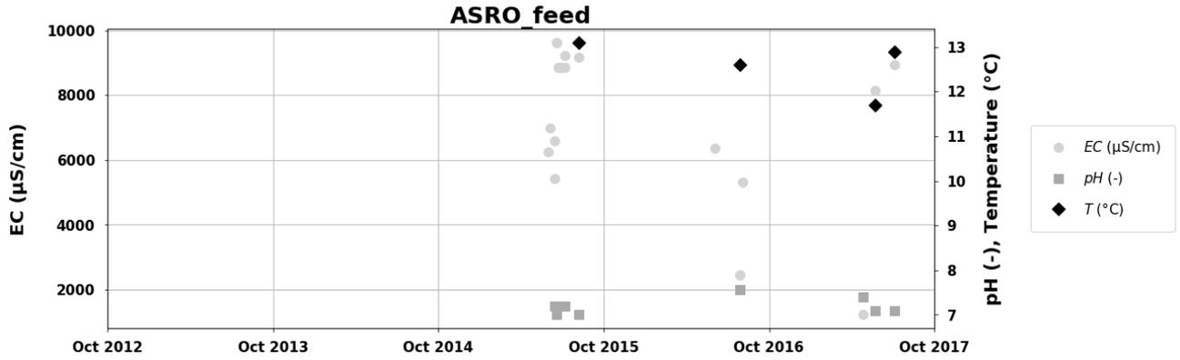
Figure 40: Electrical conductivity (EC in µS/cm), pH (-), and temperature (Temp in °C) of brackish groundwater intercepted to feed the ASRRO-system.
