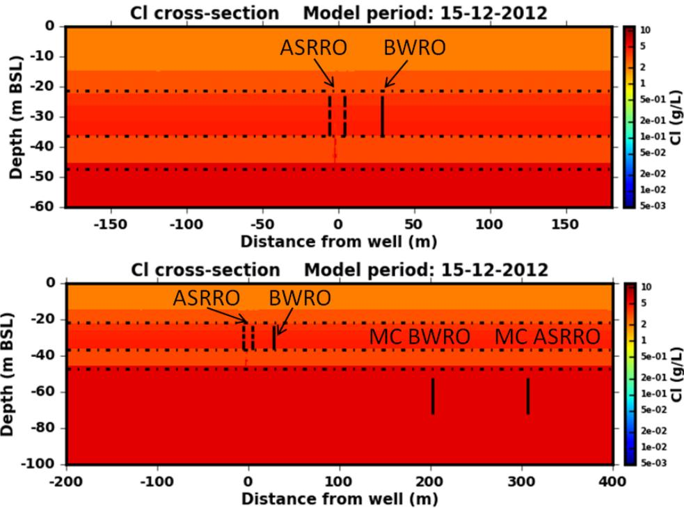
Figure 26: Initial chloride concentrations (15 December 2012) for cross-sections through the ASSRO wells (AW1 and AW2), both near the ASRRO (top) and an overview including membrane concentrate injection wells (bottom).
