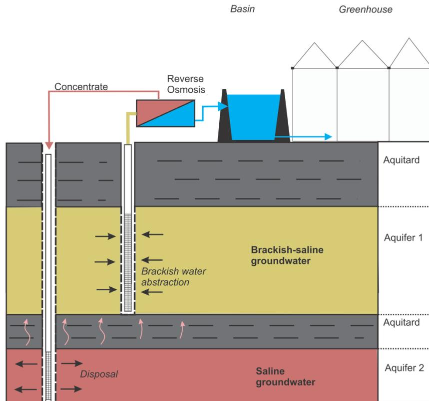
Figure 2: Use of brackish water reverse osmosis (BWRO) accompanied by concentrate disposal in the area.
