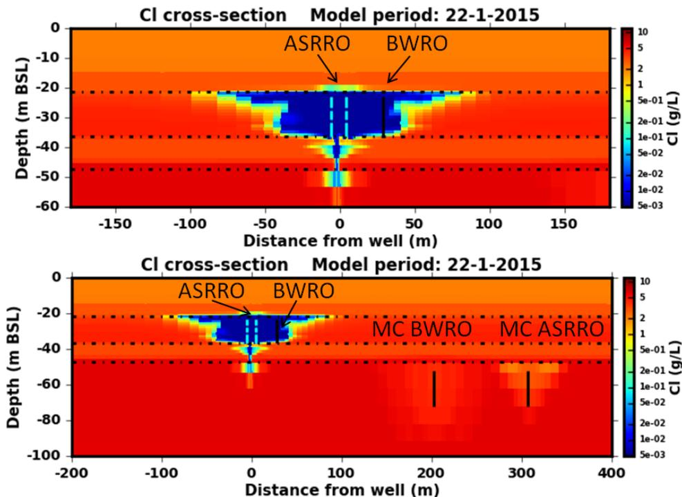
Figure 27: Modelled chloride concentrations after a prolonged period of infiltration (22 January 2015) for cross-sections through the ASSRO wells (AW1 and AW2), both near the ASRRO (top) and an overview including membrane concentrate injection wells (bottom).
