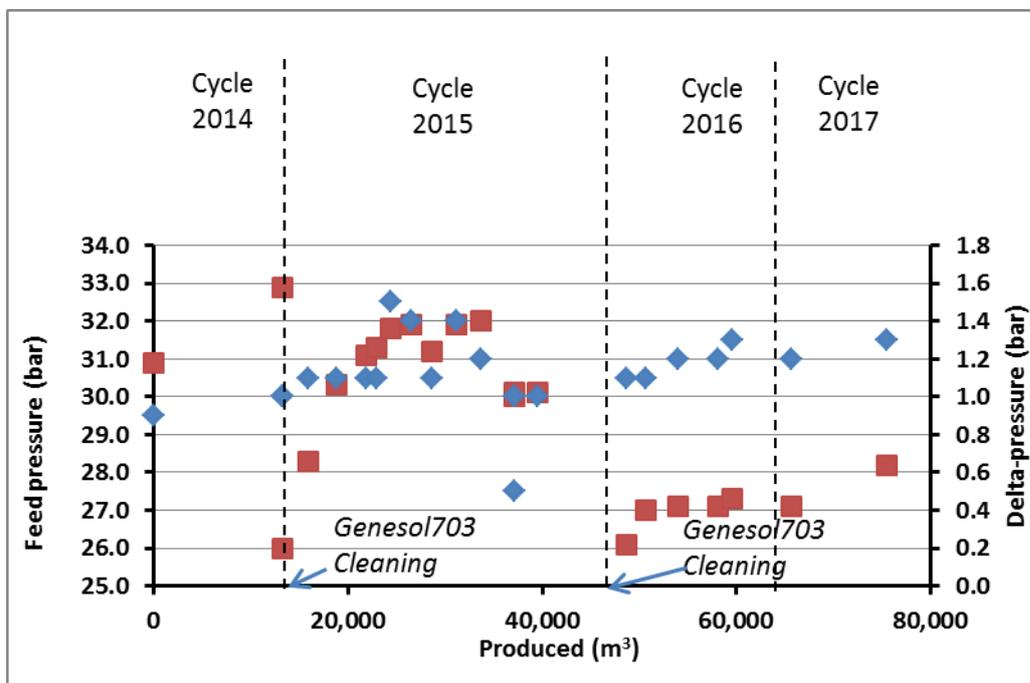
Figure 20: Feed pressure (red) and delta-pressure (blue) between feed and reject side for the BWRO-plant.
