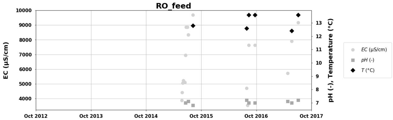
Figure 37: Electrical conductivity (EC in µS/cm), pH (-), and temperature (Temp in °C) of brackish groundwater intercepted to feed the BWRO-system.
