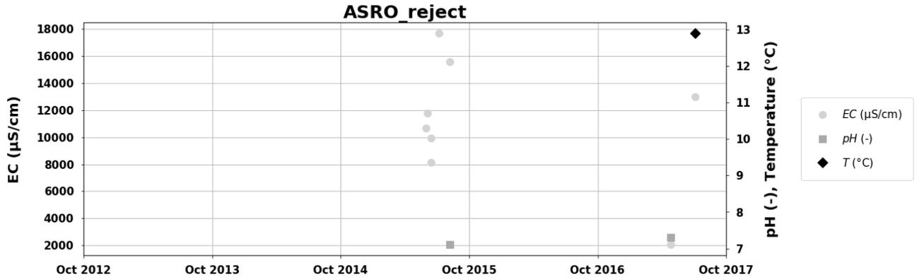
Figure 46: Electrical conductivity (EC in  $\mu\text{S}/\text{cm}$ ), pH (-), and temperature (Temp in  $^{\circ}\text{C}$ ) of brackish groundwater rejected by the ASRRO-system.
