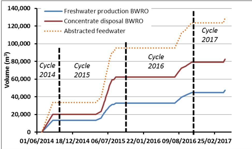
Figure 15: Freshwater production and concentrate disposal by the BWRO-plant.
