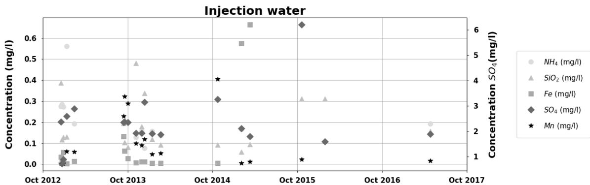
Figure 32: Concentrations of NH<sub>4</sub>, SiO<sub>2</sub>, Fe, SO<sub>4</sub>, and Mn in the freshwater used for infiltration at ASRRO Westland.
