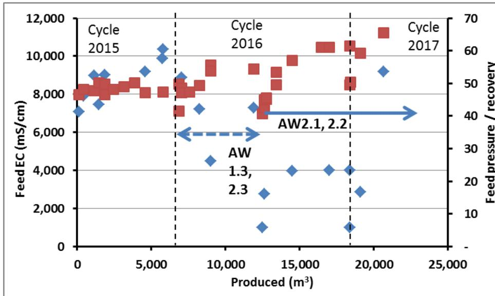
Figure 18: The feed pressure – recovery ratio (red) and the observed ECs (blue) of the feedwater during sampling at the ASRRO plant.
