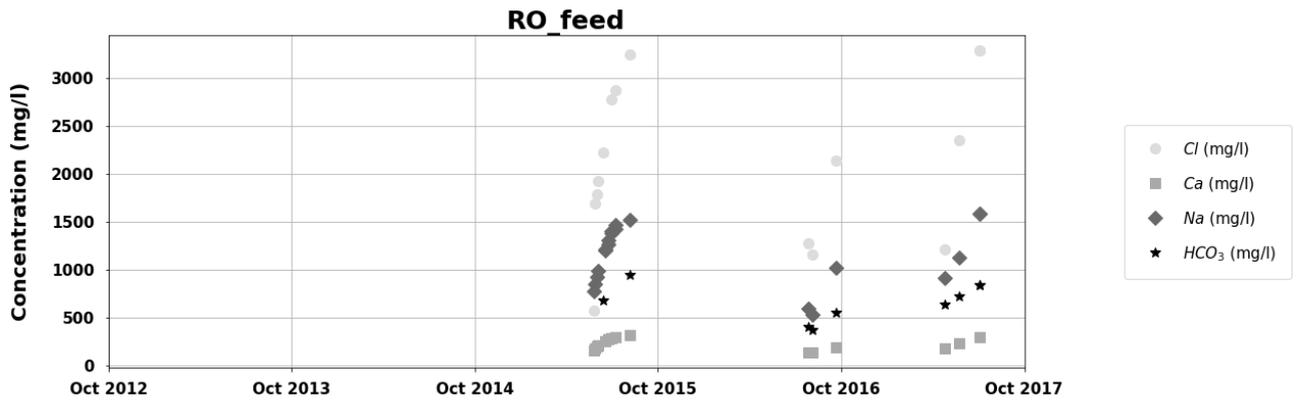
Figure 38: Concentrations of Cl, Ca, Na, and HCO<sub>3</sub> in brackish groundwater intercepted to feed the BWRO-system.
