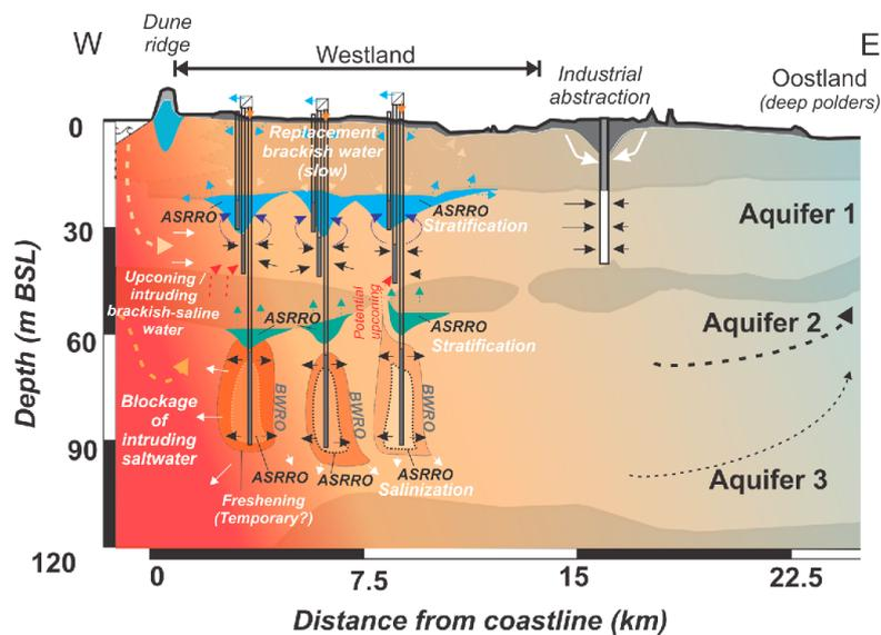
**Figure 10.** Overview of the integral impacts of ASRRO (and BWRO) on the regional salinity distribution in the Westland study area in a west-east cross-section. Local impact include salinization (BWRO) and stratification (ASRRO), while regionally saltwater intrusion (Aquifer 1) and brackish water outflow are the main phenomena, having the most negative impact in the BWRO scenario.
