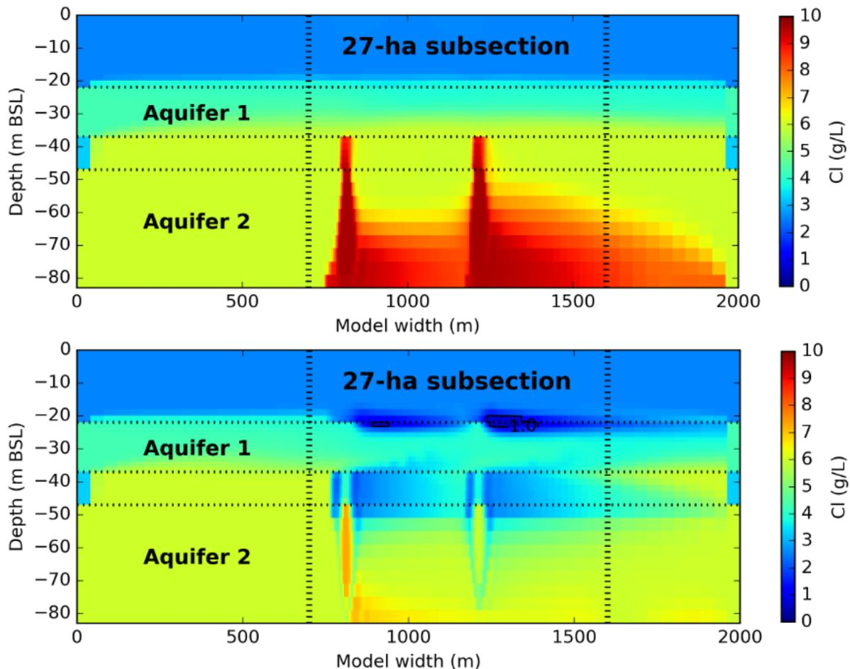
Figure 34: Cross-section of the average concentrations of chloride in the Westland groundwater system after 30 years with typical use of BWRO (current situation), and ASRRO (approach developed in DESSIN).
