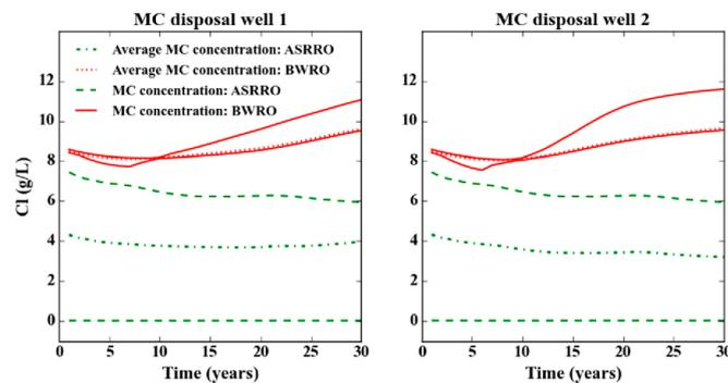
**Figure 7.** Range of MC concentrations with time of water injected by MC disposal well 1 and MC disposal well 2, for ASRRO and BWRO; and the yearly averaged MC concentration of each MC disposal well for both scenarios.
