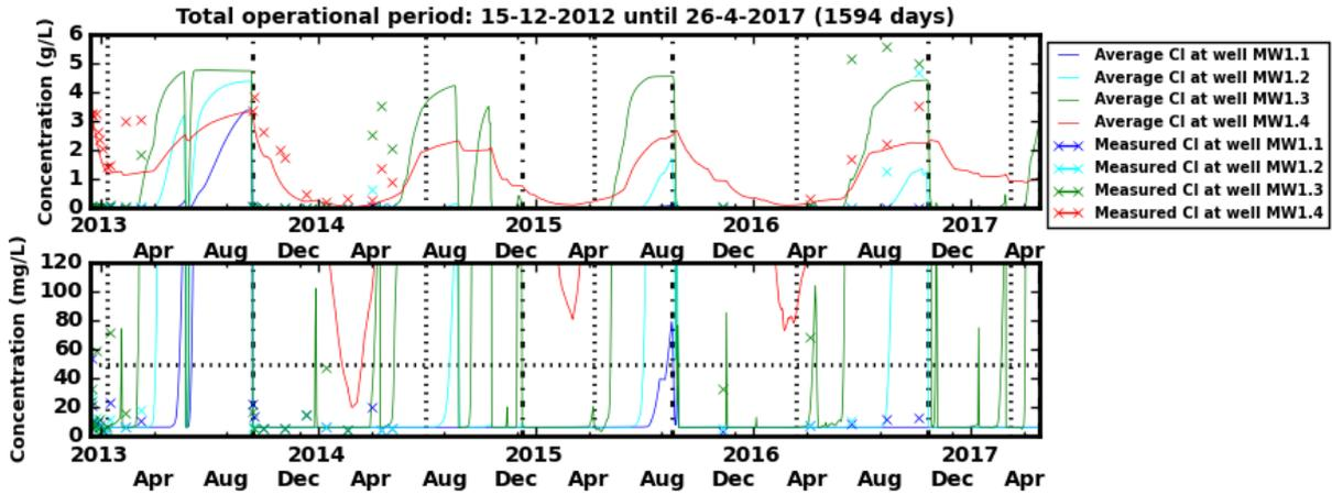
Figure 51: Measured (crosses) and modelled (solid lines) chloride concentration in water in the different well screens of the monitoring well (MW1) at Westland from 15 December 2012 until 26 April 2017. The black dotted and dashed vertical lines indicate the start of the infiltration and recovery period respectively. The horizontal dashed line in the bottom graph represents the maximum allowable concentration limit of chloride upon abstraction.
