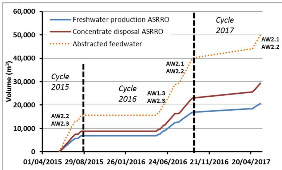
Figure 13: Freshwater production and concentrate disposal by the ASRRO-plant. The ASRRO wells feeding the ASRRO-plant during the various stages are indicated.
