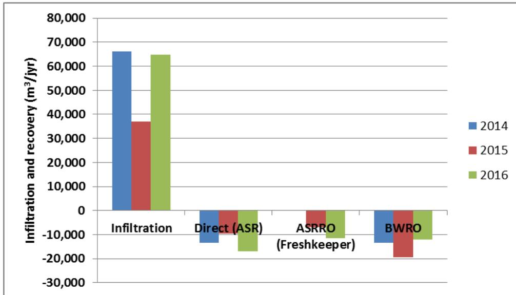
Figure 23: Infiltration, direct recovery (unmixed), production of the ASRRO-plant (brackish water recovered with Freshkeeper), and production of the BWRO plant.
